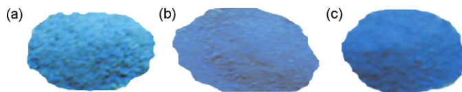
Fig. 9. Color for 0.01 mol (a), 0.05 mol (b) and 0.1 mol (c) of \text{Co}^{2+} at 1200^\circ\text{C} using urea as a fuel.
